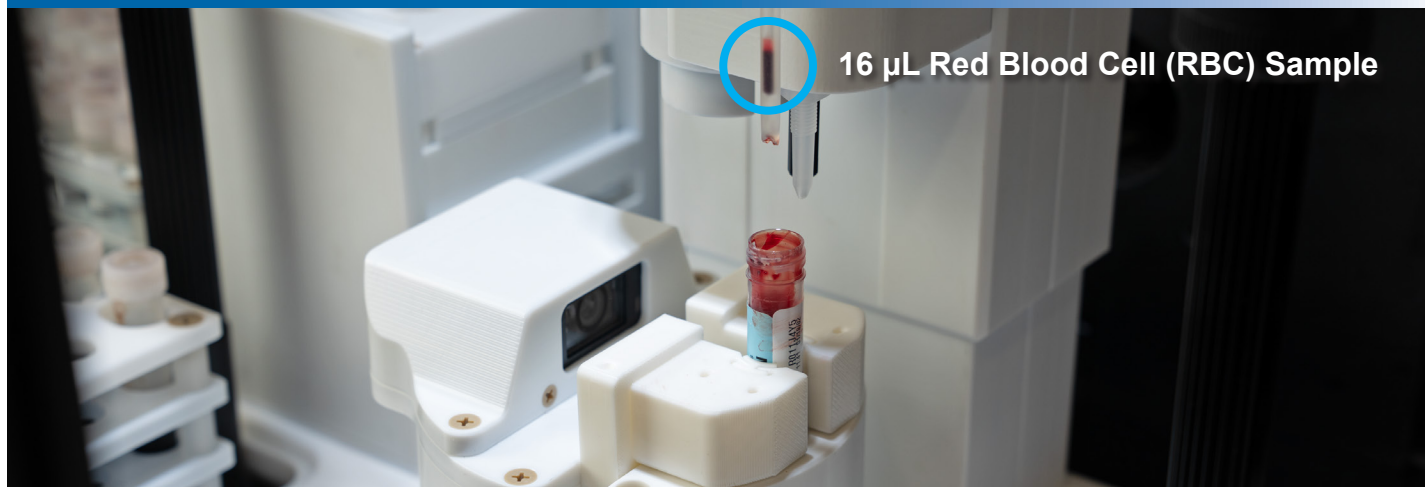
Figure 2. TRAXStation Clinical takes up a 16 µL RBC aliquot for automated preparation to a final volume of 4000 µL.
